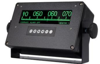
The received information is also converted into industry standard NMEA 0183 data and output as RS422 serial data.
